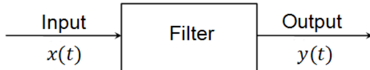
Figure 2.8 – Block diagram of a filter with one input and one output
